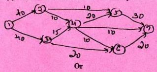
(b) Using a labelling algorithm for flow augmenting path, find the maximum flow for the network.
